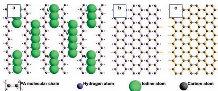
Figure 48. (a) Structural model of the iodine-doped PA. (b) Hypothetical molecular model of the specimen formed on the way to the dehydrogenation reaction from the iodine-doped PA film shown in Figure 48a. (c) Hexagonal carbon bond network formed at 800 °C after passing through the model shown in Figure 48b.
